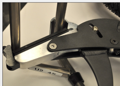
Adjust the "rear end" by screwing in or out until the FreeWheel fit the footrest. See page 6.
